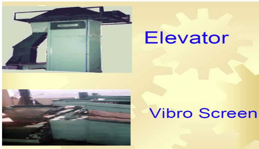
Figure 7: Elevator and Vibro screen for refinement section
