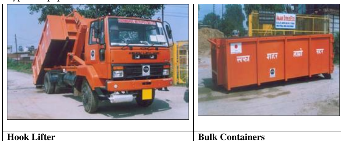
Picture 6: Type of Equipment /Vehicle for Transfer Station
